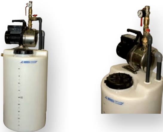
Filling and mixing vessels for the brine, 100 litres (pump 1 phase 230 Volts)
